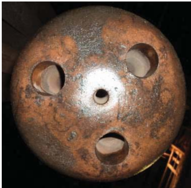
Figure 2 – Photo of Tip with 3 Angled Nozzles and 1 Small Central Nozzle.
