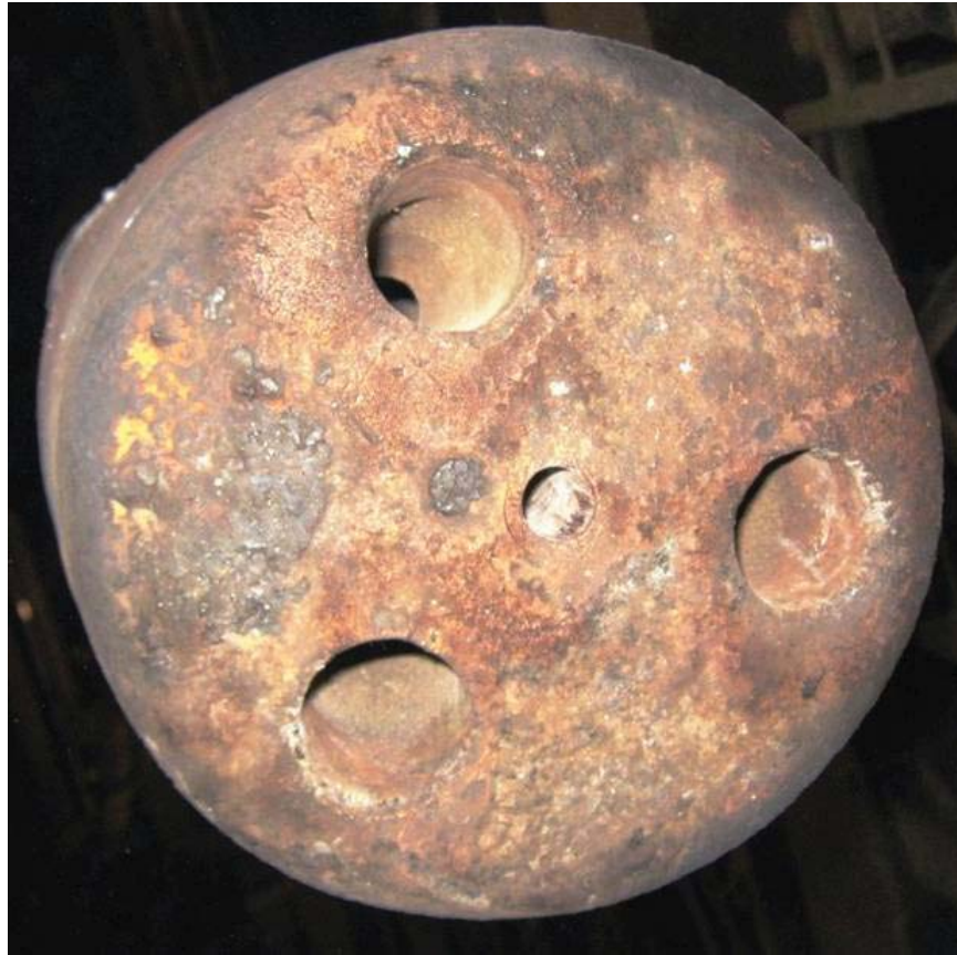
Figure 5 – 3-Nozzle Tip with Damage Around Nozzle Exits Due To Over-expanded Jet.
