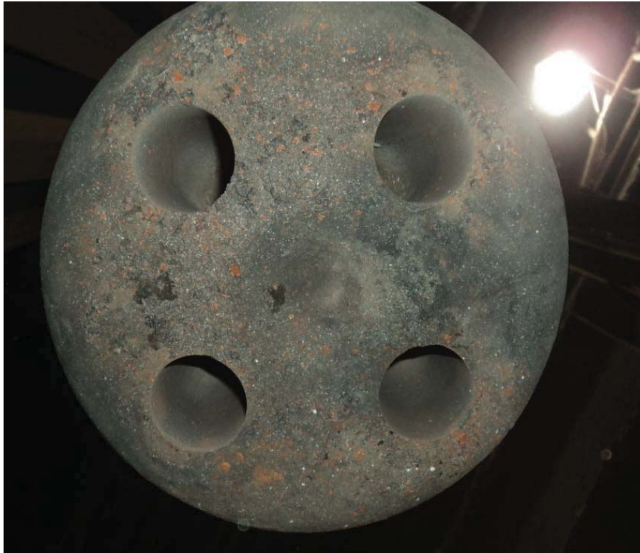
Figure 10 – 4-Nozzle Tip Face from Steel Plant 1 with 247 Heats.
